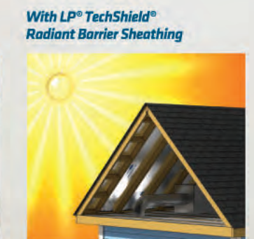
LP® TechShield® Radiant Barrier Sheathing blocks up to 97% of the radiant heat in the panel from radiating into the attic.
